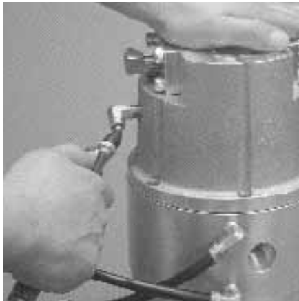
Step 8. Figure 8 To lift the liquid chamber away from the center section, apply 1.0 bar (15 psig) of air pressure, via a rubber tipped air nozzle into the brass elbow located at the top of the liquid chamber.
