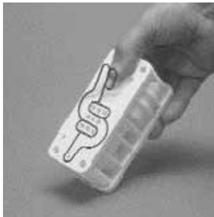
Step 3. Figure 3 Inspect air valve gasket and replace if necessary.
