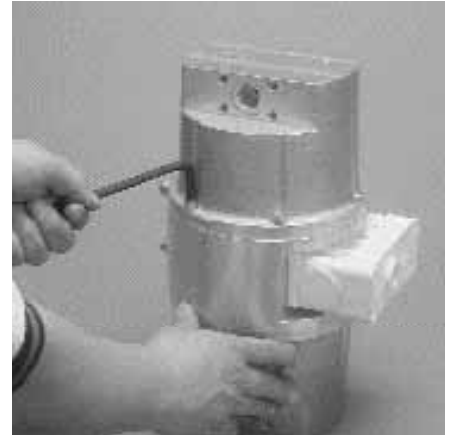
Step 7. Figure 7 Using a 6 mm (1/4") hex head wrench, remove the liquid chamber bolts that connect the liquid chamber to the center section.
