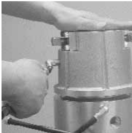
Step 9. Figure 9 The air pressure will force the liquid chamber away from the power piston to allow for easy removal. To remove the opposite liquid chamber repeat Step 9.
