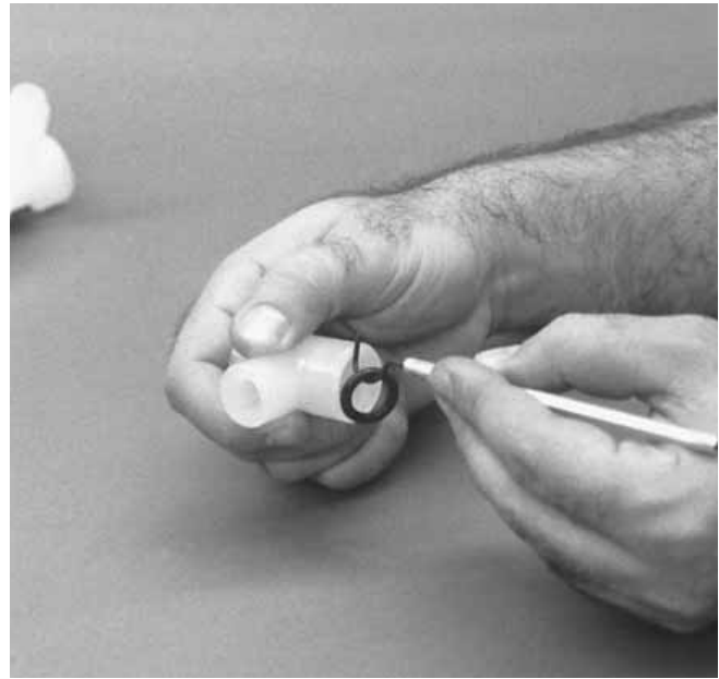
Step 9. Figure 9 Carefully remove tee-section o-ring. Inspect o-ring for wear and replace with genuine Wilden parts if necessary.
